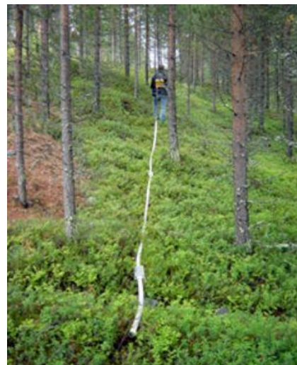
Figure 2. Example of 30 MHz rough terrain GPR antenna.
