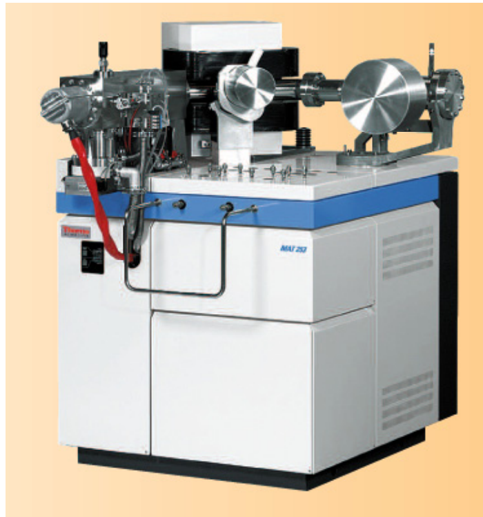
Figure 1. Mass spectrometer able to measure clumped isotopes. The instrument has four collectors and sensitive amplifiers that allow measuring the species at the 44-49 masses.
